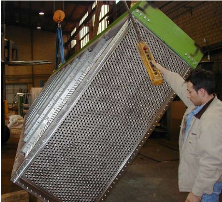
FIGURE 1 Zeron 100 heat exchanger supplied to BOC Cantarell to handle seawater with a high suspended solids content.
