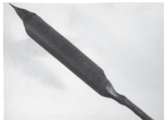
Fig. 2. 316L round-bar 3/4 inch in diameter exposed to 1800°F in air atmosphere. 316L is suggested to be used only to 1500°F due to scaling. In contrast, its melting point is 2540°F.
