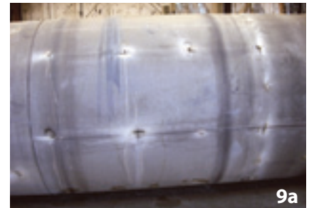
Fig. 6. U-type radiant tube made primarily from RA330 alloy but with RA333 for 2-foot section most prone to metal-dusting attack.
